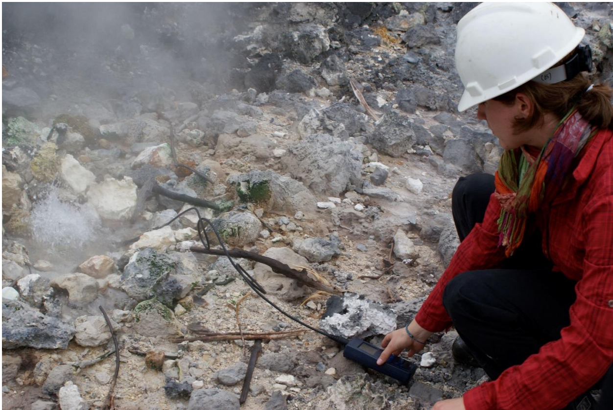
Fluid property measurements in boiling hot springs of Ulubelu geothermal field in Indonesia in 2010
